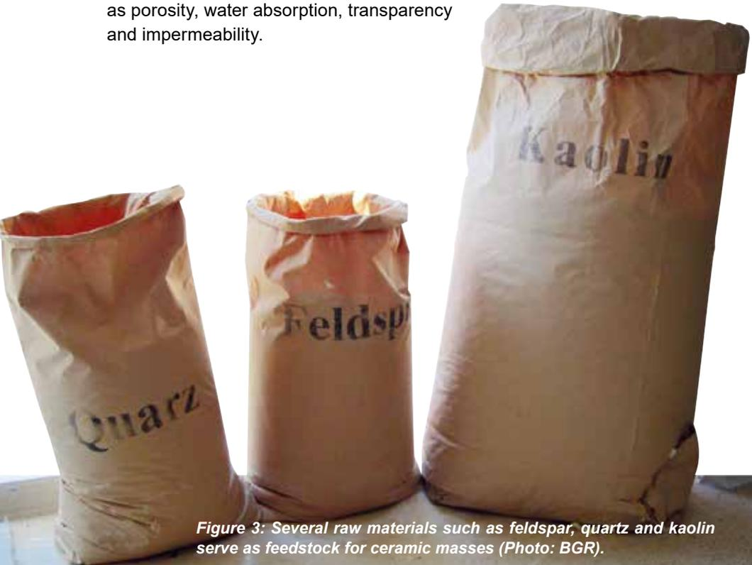
*Figure 3: Several raw materials such as feldspar, quartz and kaolin serve as feedstock for ceramic masses (Photo: BGR).*
