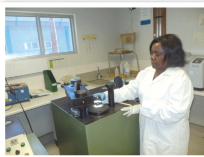
Preparation of pressed pellets with the hydraulic press
