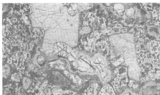
Fig. 10: Photomicrograph of gabbro xenolith sample DRK-72, showing primary igneous minerals clinopyroxene (clear), olivine (high relief with cracks accentuated by dusting of secondary magnetite), and plagioclase (showing patchy turbid alteration). Olivine in contact with plagioclase shows extensive reaction and the development of a multiple corona, while the grain in the centre of the photograph is unaffected where it is in contact with clinopyroxene. Width of photograph is 6.5 mm.
