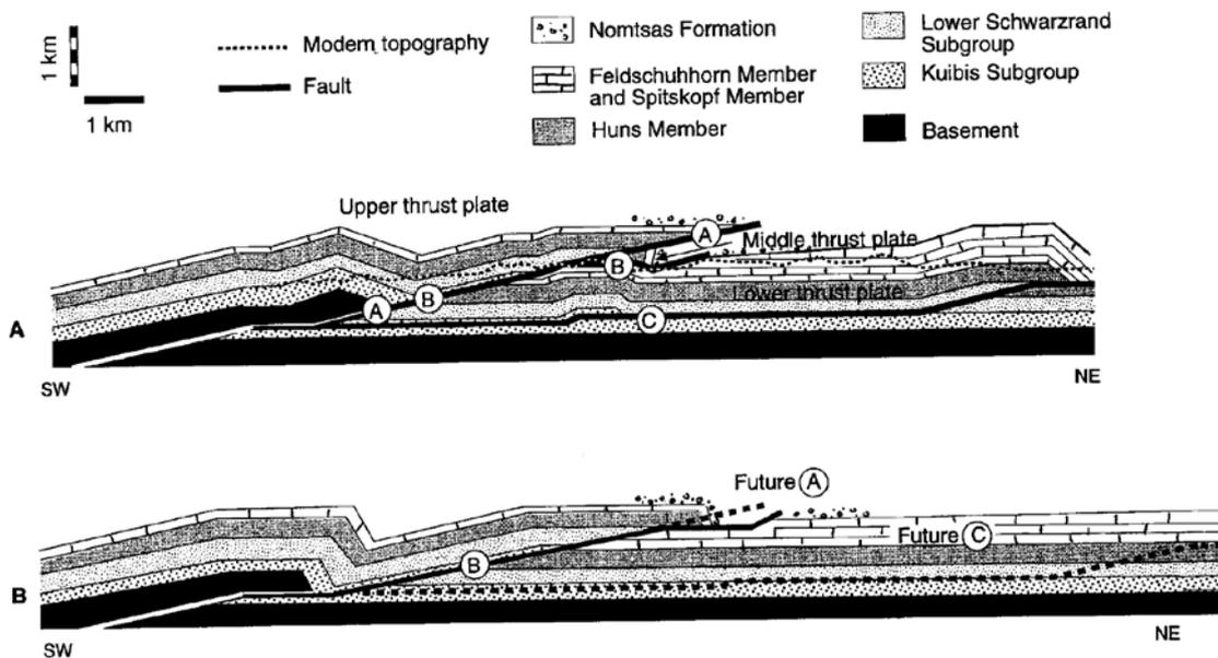
**Figure 7:** a. Cross-section showing the lower, middle and upper thrust plates. Location of cross-section shown in figure 1. b. Partially restored cross-section showing geometry prior to movement along fault C and splay A. Note that the lower Schwarzrand Subgroup includes the Nudaus Formation and the Nasep Member.
