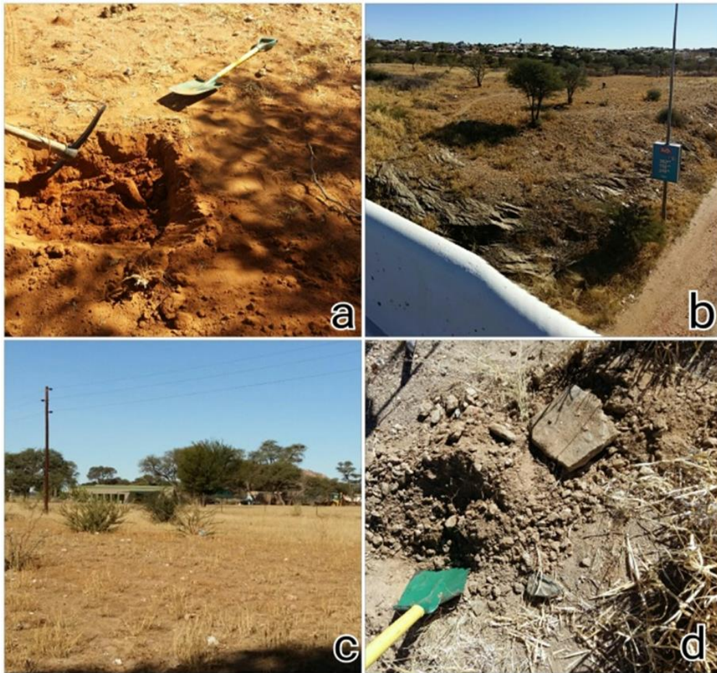
Figure 4. Site images: (a) Boring at Rehoboth North; (b) Acacia sampling site; (c) Location of housing construction at Rehoboth South; (d) Boring location in Acacia underlain by mica schist and quartz
