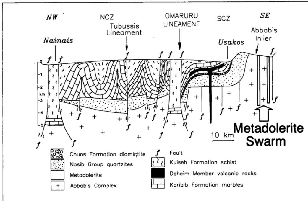
**Figure 3:** Cross-section through the Central Zone of the Damara Orogen showing basement faults and metadolerite swarm in the underlying mid-Proterozoic basement (after Steven, 1993). Note feeder to Daheim Member volcanic rocks.
