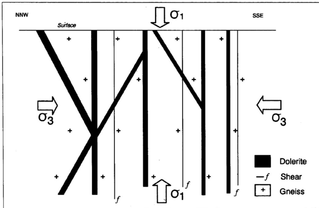
**Figure 2:** Cross-section showing orientation of metadolerites in the Abbabis Inlier and indicated stress field at the time of their emplacement
