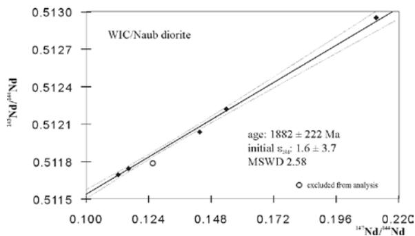
**Figure 8:** Sm-Nd errorchron diagram of samples from of the WIC and Naub diorite (stippled lines mark error envelope)
